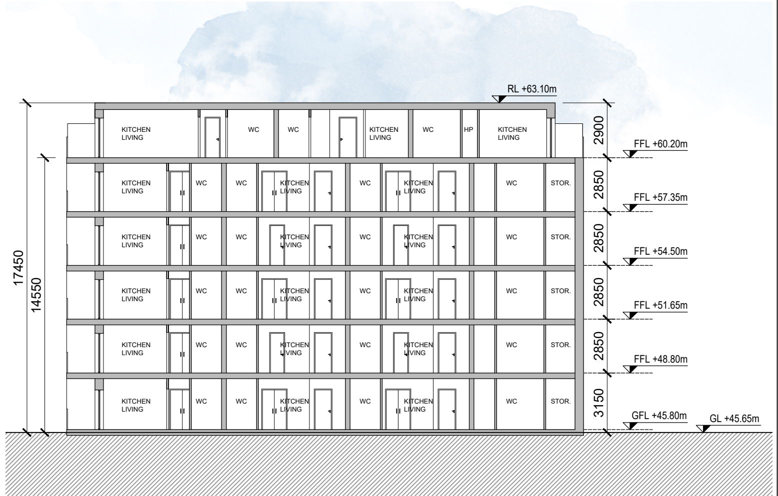
This architectural elevation drawing shows a building facade with various height markers and level indicators. The drawing includes a ground line (GL) at +45.65m and a ground floor level (GFL) at +45.80m. The building has a total height of 17,450mm, with a base section of 3,150mm and a main section of 14,550mm. The main section is divided into four floors, each 2,850mm high, with a top section of 2,900mm. The building is divided into two main sections: a left section with a brown facade and a right section with a dark brick facade. The left section has a total height of 15,000mm, and the right section has a total height of 15,000mm. The building is surrounded by trees and a sky with birds. A north arrow is located at the bottom center of the drawing. Key height markers and level indicators include: RL +63.10m (Roof Level) FFL +60.20m (Finished Floor Level) FFL +57.35m (Finished Floor Level) FFL +54.50m (Finished Floor Level) FFL +51.65m (Finished Floor Level) FFL +48.80m (Finished Floor Level) GFL +45.80m (Ground Floor Level) GL +45.65m (Ground Level) The drawing also includes a north arrow and a scale bar indicating 1:100.
